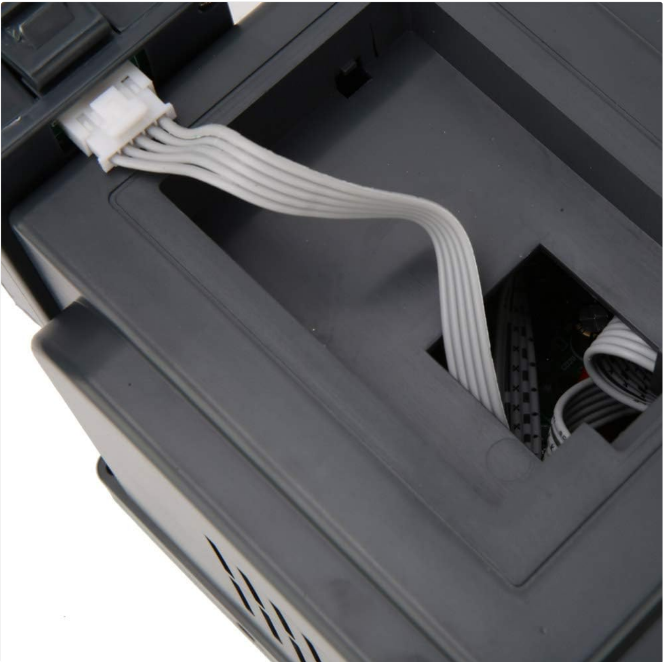
Figure 5.1: Internal ribbon cable connection, illustrating modular design for control panel. This area should only be accessed by qualified technicians.
