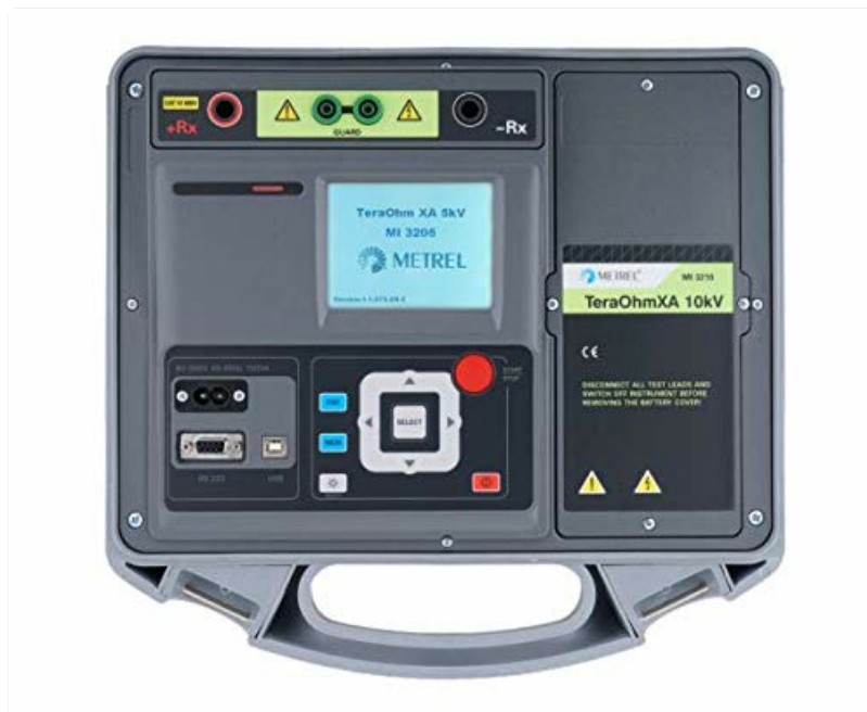
Figure 3: Top panel of the MI 3210 showing connection ports.
