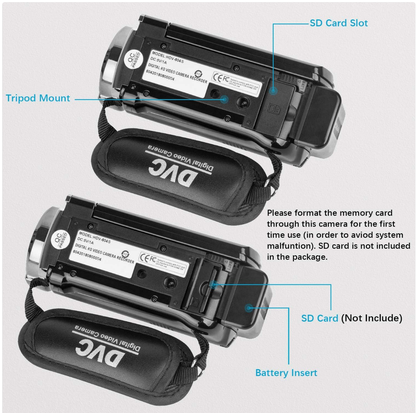
Figure 3: Location of battery and SD card slots.
