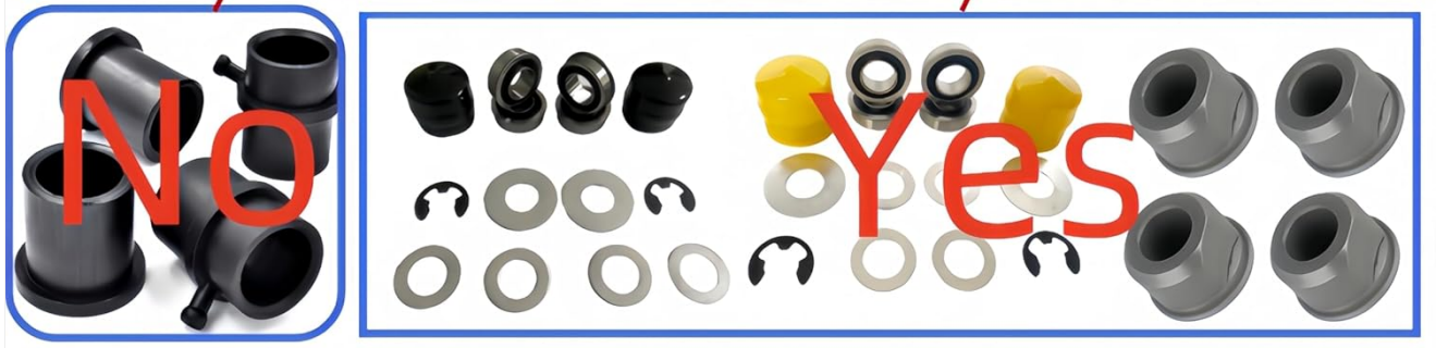
Image 2.1: Visual guide for determining compatibility by measuring the outer diameter of the lawn mower wheel hub liner or bearing hole. The kit is suitable for wheels with a 1-1/2 inch (38.1mm) outer diameter bearing hole.
