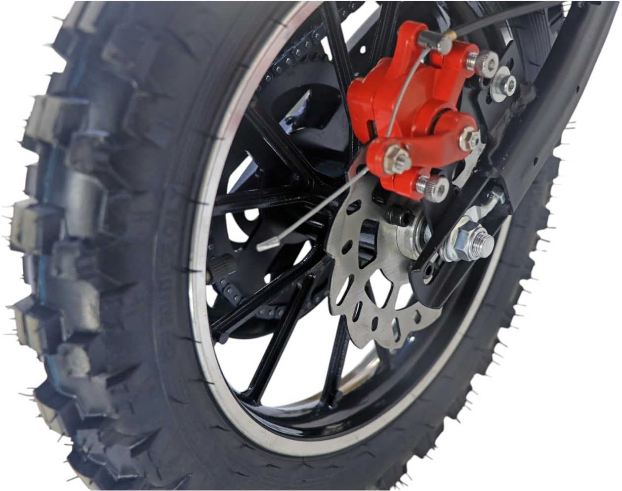
Image 6.1: The rear wheel assembly, highlighting the disc brake and knobby tire for off-road traction.
