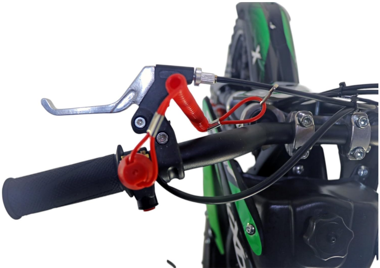
Image 2.1: The safety leash connected to the kill switch on the handlebar, designed for emergency stops.
