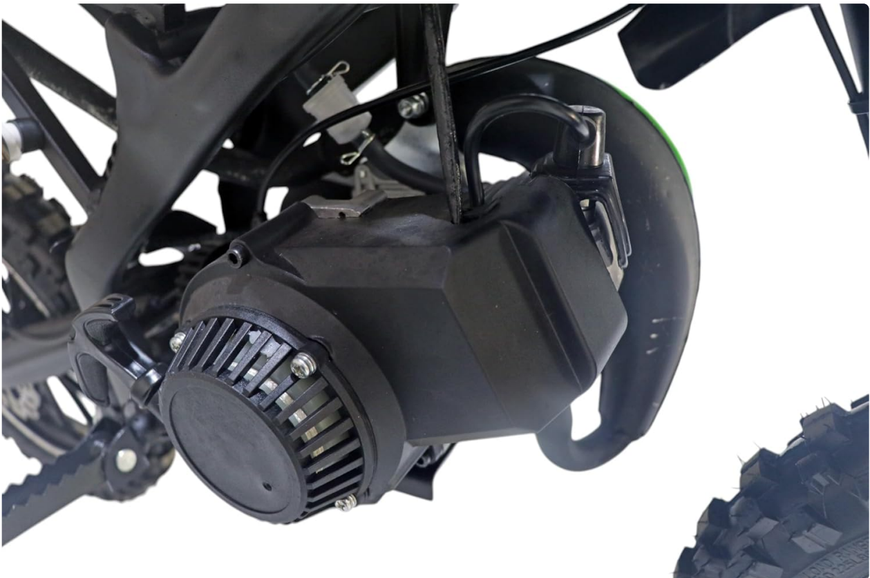
Image 5.1: The 49ccm 2-stroke engine with the pull starter mechanism.
