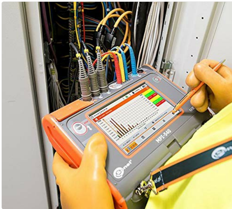
Figure 3.1: An electrician using the MPI-540 to perform measurements within an electrical panel, demonstrating proper probe connection.
