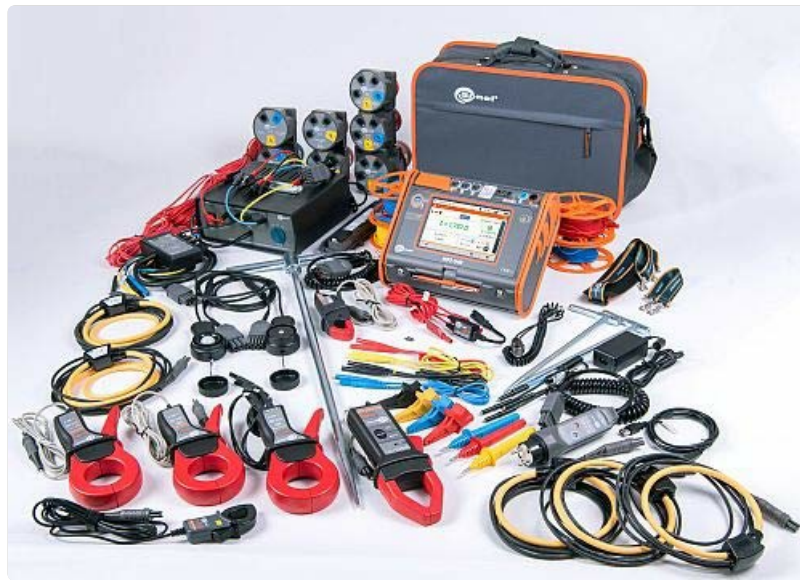
Figure 2.1: The MPI-540 meter shown with its comprehensive set of accessories, including various probes, clamps, and cables.
