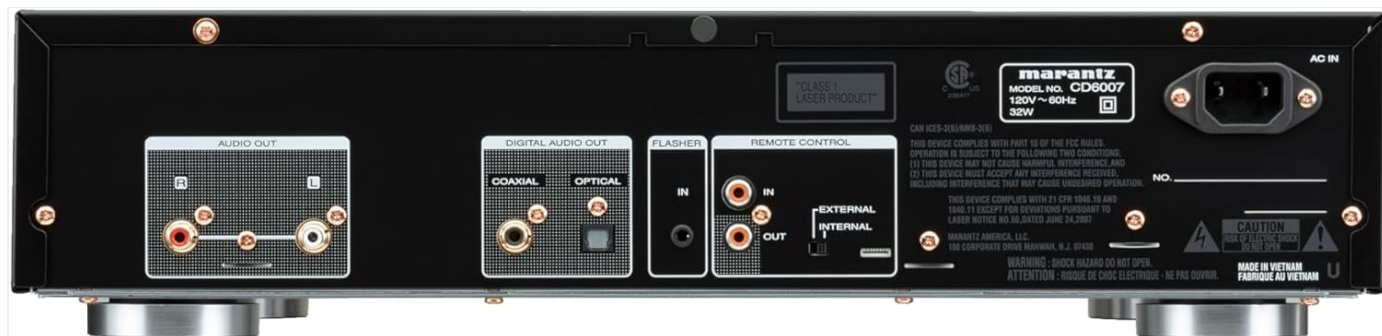
Figure 1: Rear Panel Connections. This image displays the rear panel of the Marantz CD6007, highlighting the analog audio output (RCA L/R), digital audio outputs (coaxial and optical), remote control input/output, and the AC power inlet. Proper connection of these ports is
