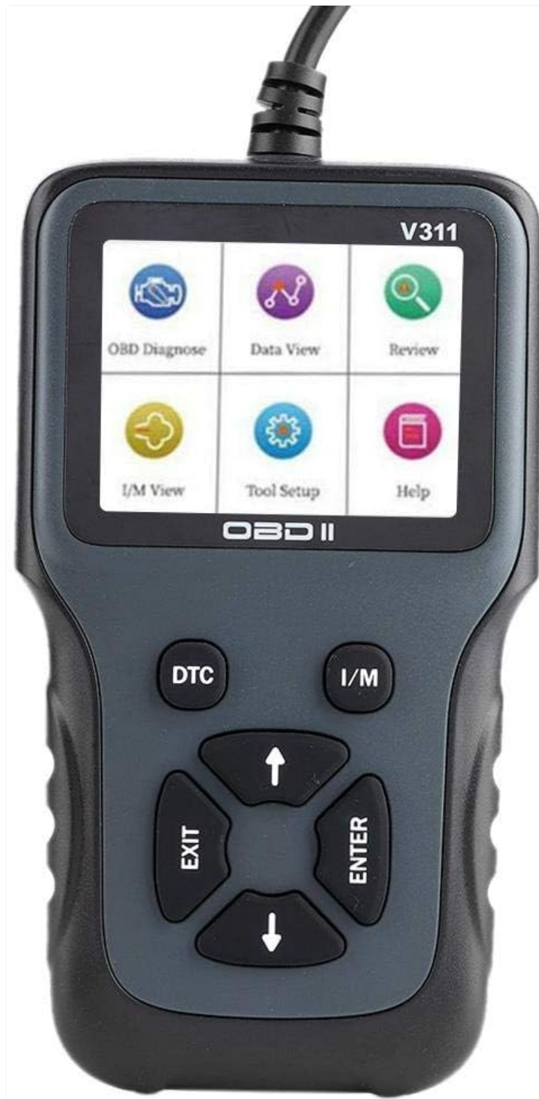
Figure 2.1: Front view of the Bigking V311 OBD2 Scanner. The device features a color screen displaying menu options like "OBD Diagnose", "Data View", "Review", "I/M View", "Tool Setup", and "Help". Below the screen are control buttons including "DTC", "I/M", "EXIT", "ENTER", and directional arrows.
