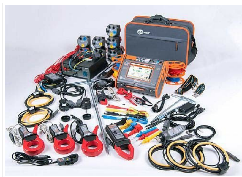
Figure 2: Sonel MPI-540 complete kit. This image displays the Sonel MPI-540 meter along with its comprehensive set of accessories, including various test leads, clamps, adapters, and a carrying bag, laid out on a white surface.
