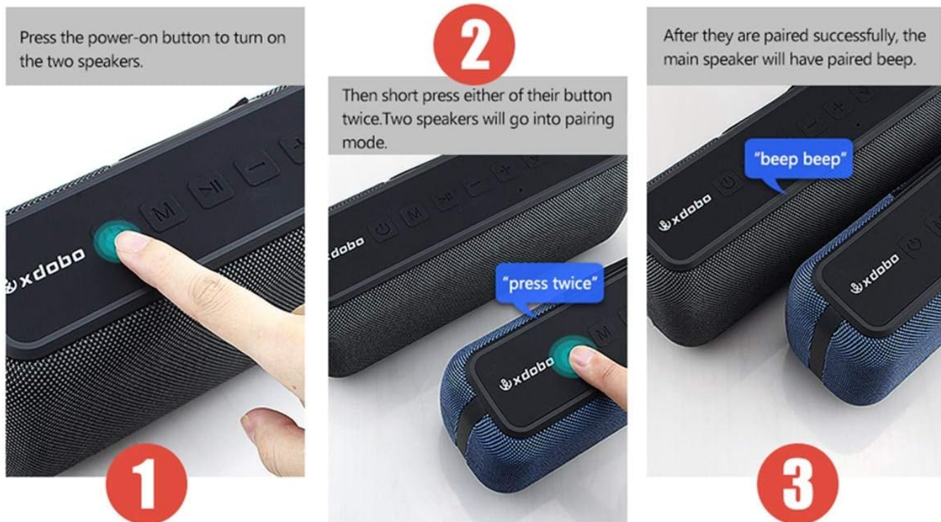
Figure 5: Steps for TWS Interconnection Operation.
