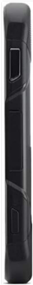
Figure 2.2.1: Side view of the Kyocera DuraForce Pro 2, illustrating the location of the SIM/MicroSD card tray and buttons.
