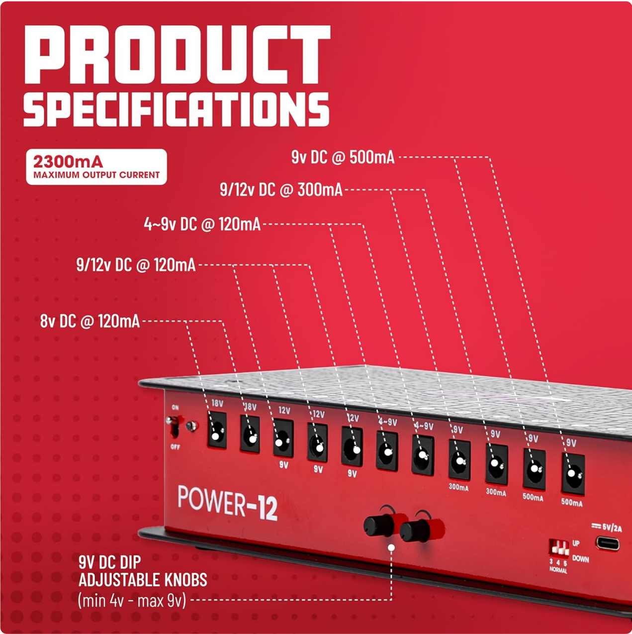
Image: Detailed diagram of the GTR-PWR-12's output specifications, including voltage and current for each port.
