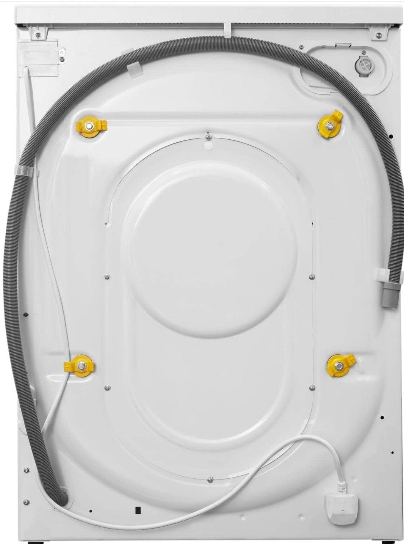
Image: The back of the washer dryer, highlighting the grey corrugated drain hose and the yellow transport bolts that must be removed before use.
