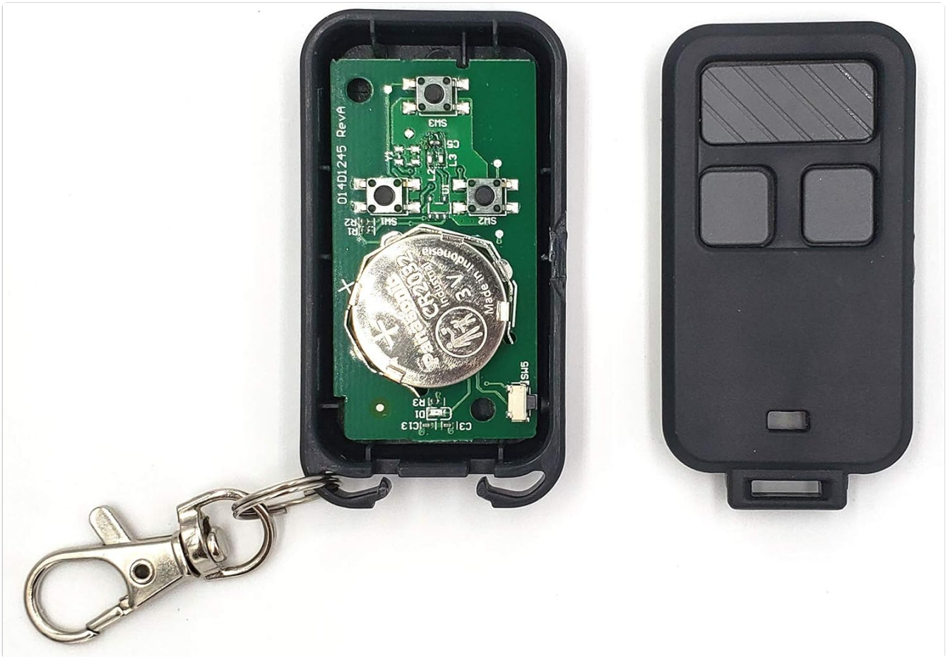
Image: The remote control opened, revealing the internal circuit board and the CR2 battery.
