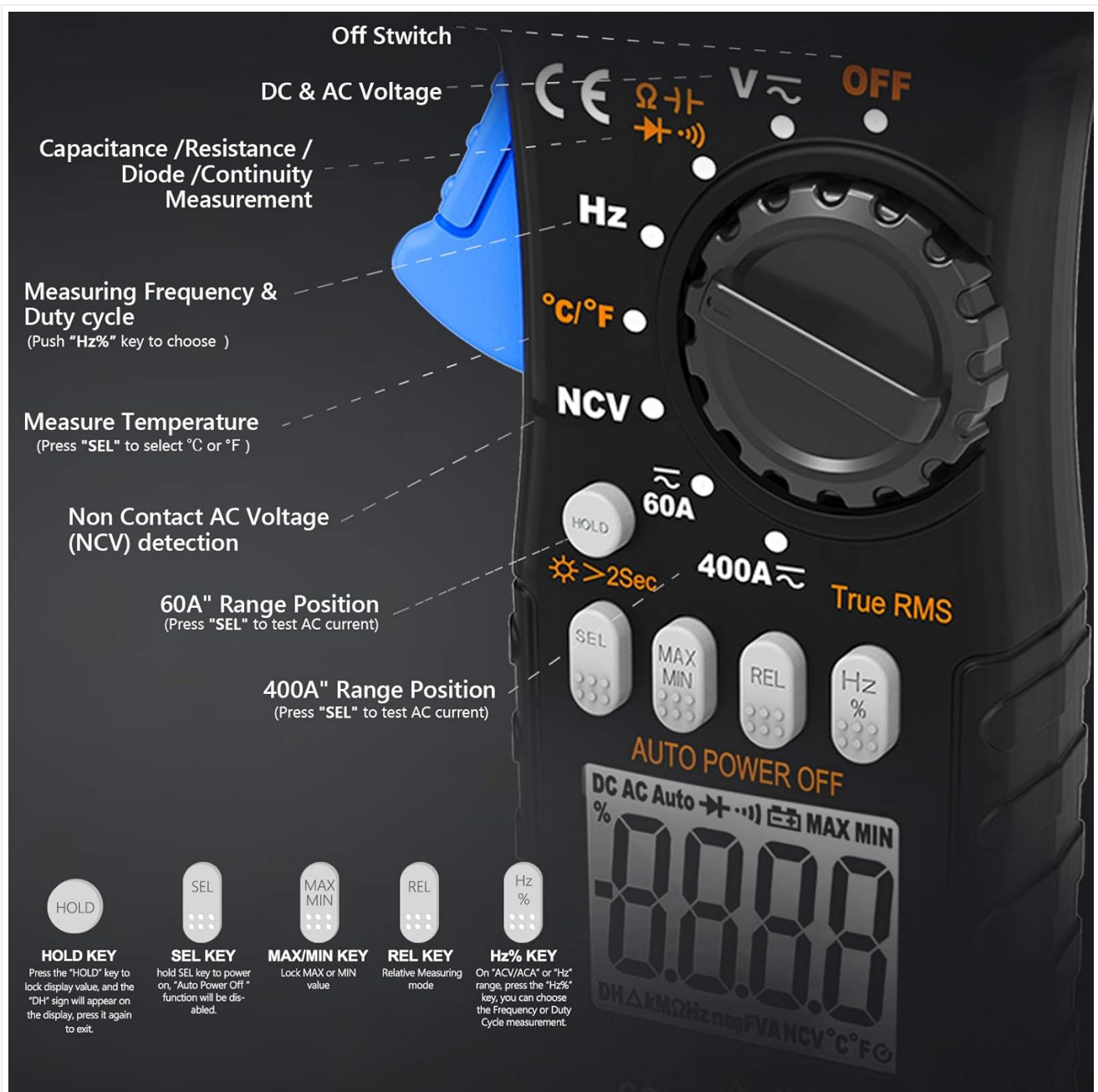
Figure 4.1: Front view of the INFURIDER YF-7200B Digital Clamp Meter with labels for controls.
