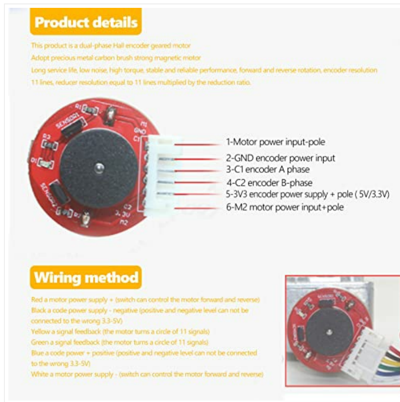
Figure 2: Detailed wiring diagram showing the 6-pin connector and corresponding functions. Pin 1: Motor power input-pole, Pin 2: GND encoder power input, Pin 3: C1 encoder A phase, Pin 4: C2 encoder B-phase, Pin 5: 3V3 encoder power supply + pole (5V/3.3V), Pin 6: M2 motor power input+pole.
