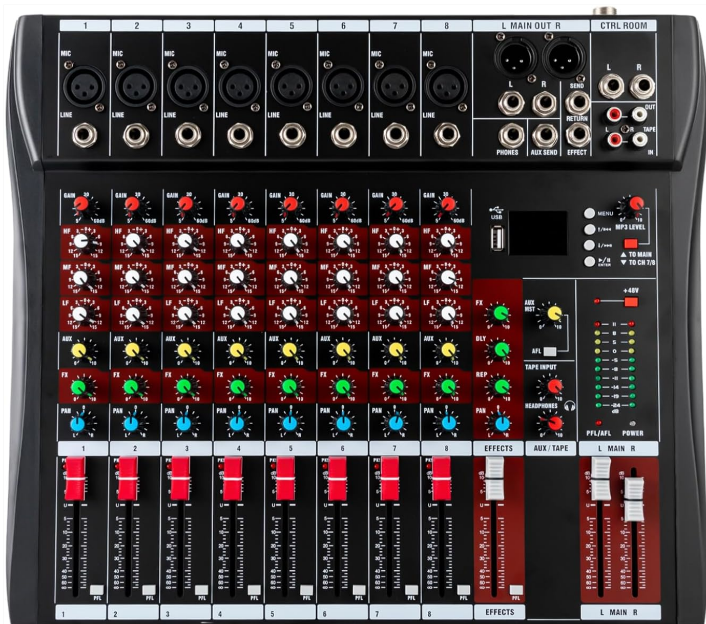
Figure 1: Overall view of the CNCEST 8-Channel Audio Mixer, showing its compact design and control layout. Dimensions are approximately 40cm (15.75in) wide, 34cm (13.4in) deep, and 3.7cm (1.46in) high.
