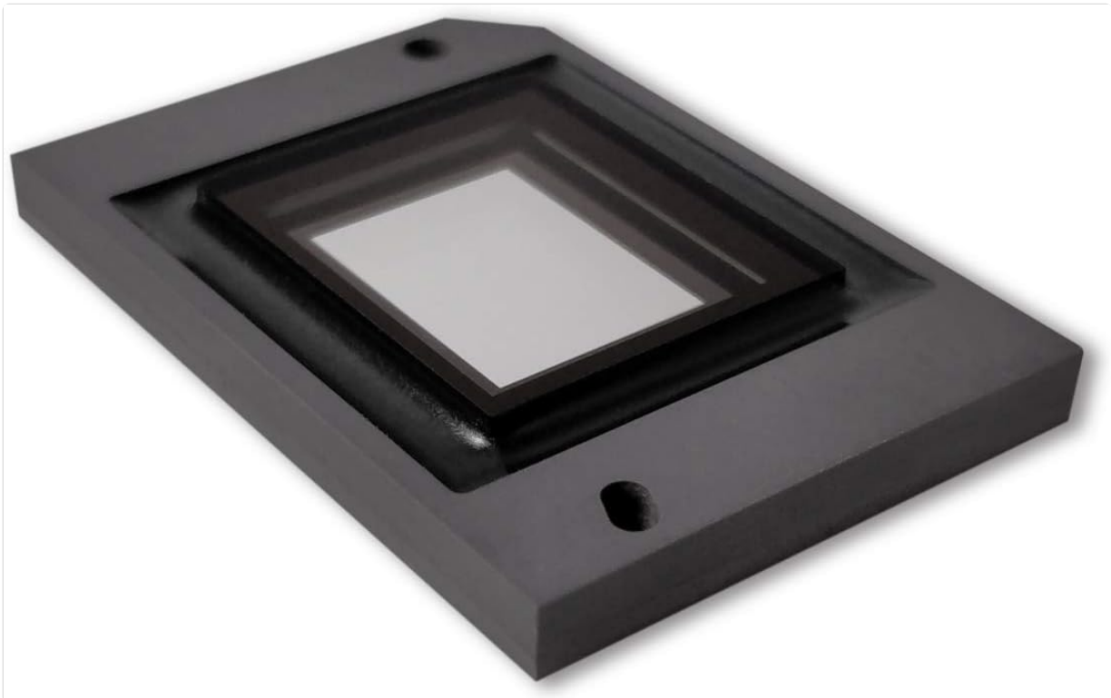
Image 4: An angled perspective of the DMD chip, providing a clearer view of the mirror array and its protective frame.
