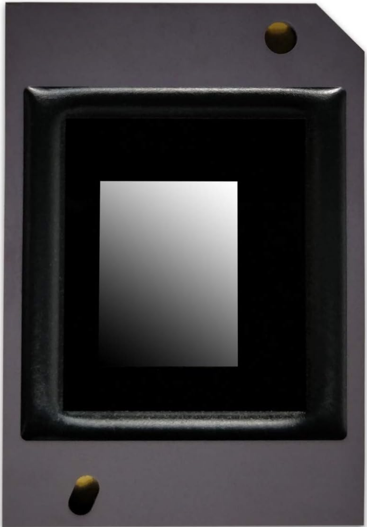
Image 3: Close-up of the DMD chip's mirror array, the delicate surface responsible for image projection. This surface should never be touched directly.
