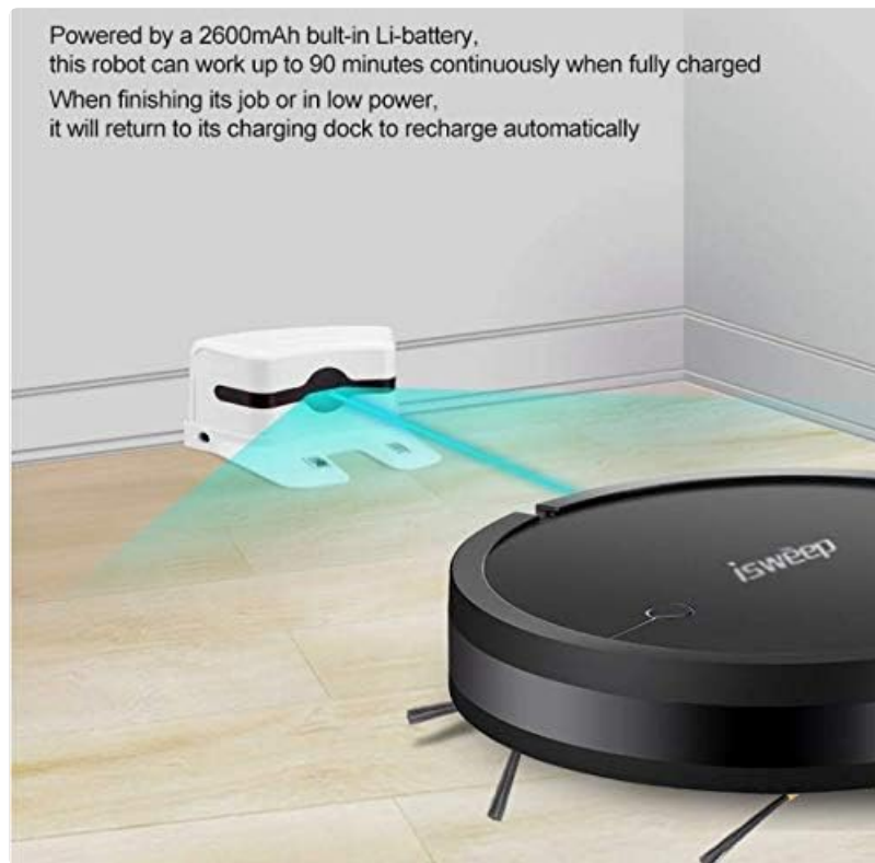
Image 5.1: The ISWEEP Robot Vacuum Cleaner automatically returning to its charging dock for recharging. The dock is placed against a wall, and the robot aligns itself for connection.
