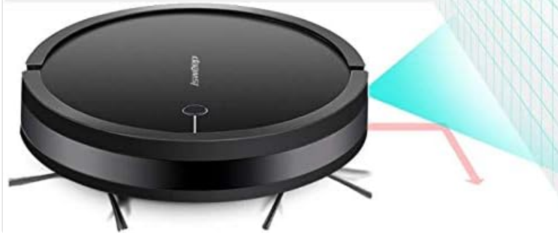
Image 7.1: The ISWEEP Robot Vacuum Cleaner illustrating its anti-collision system, which uses sensors to detect obstacles and prevent impact with furniture and walls.
