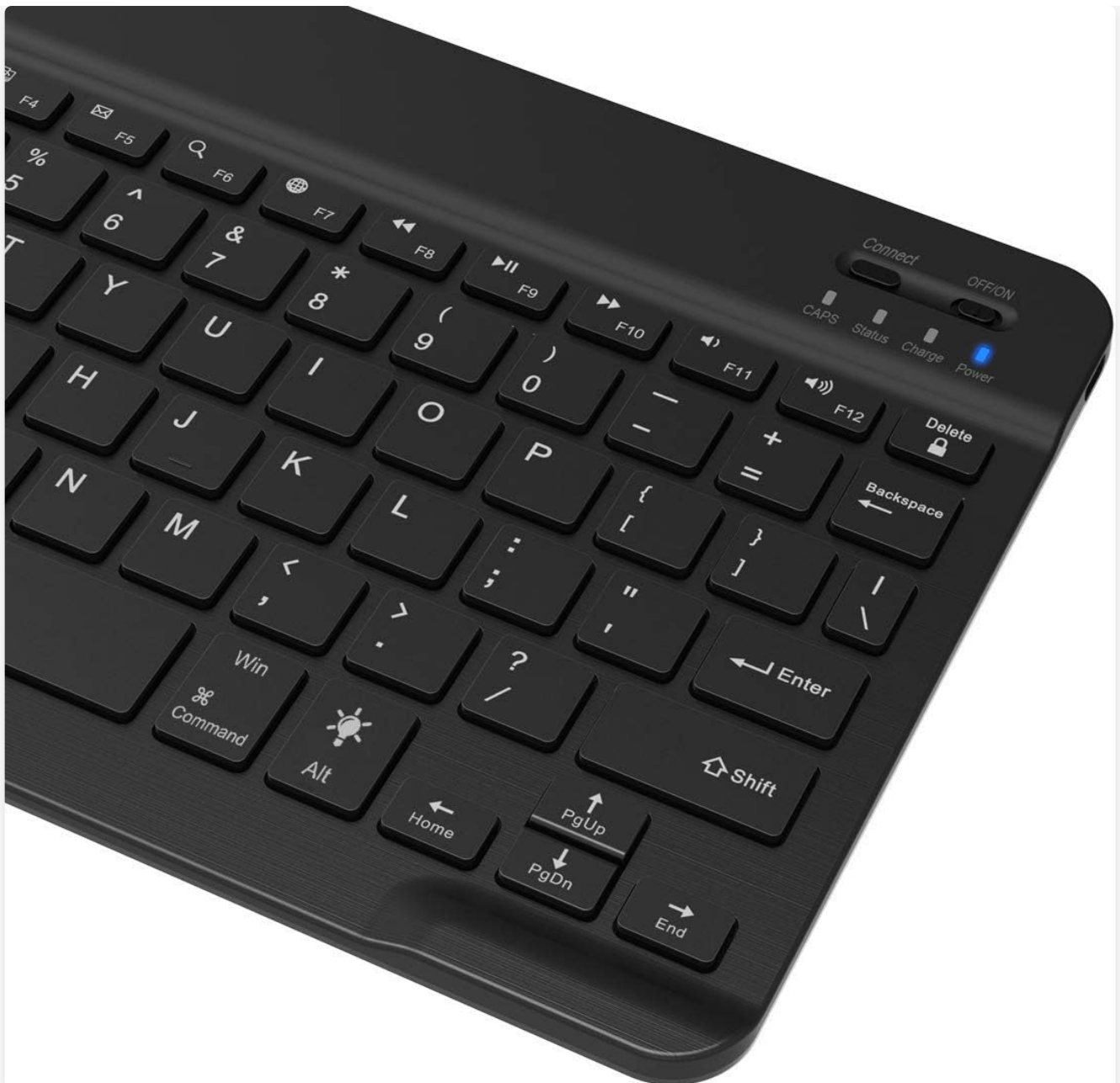
Figure 2: Close-up view of the keyboard's indicator lights, including the 'Charge' light, which indicates charging status.
