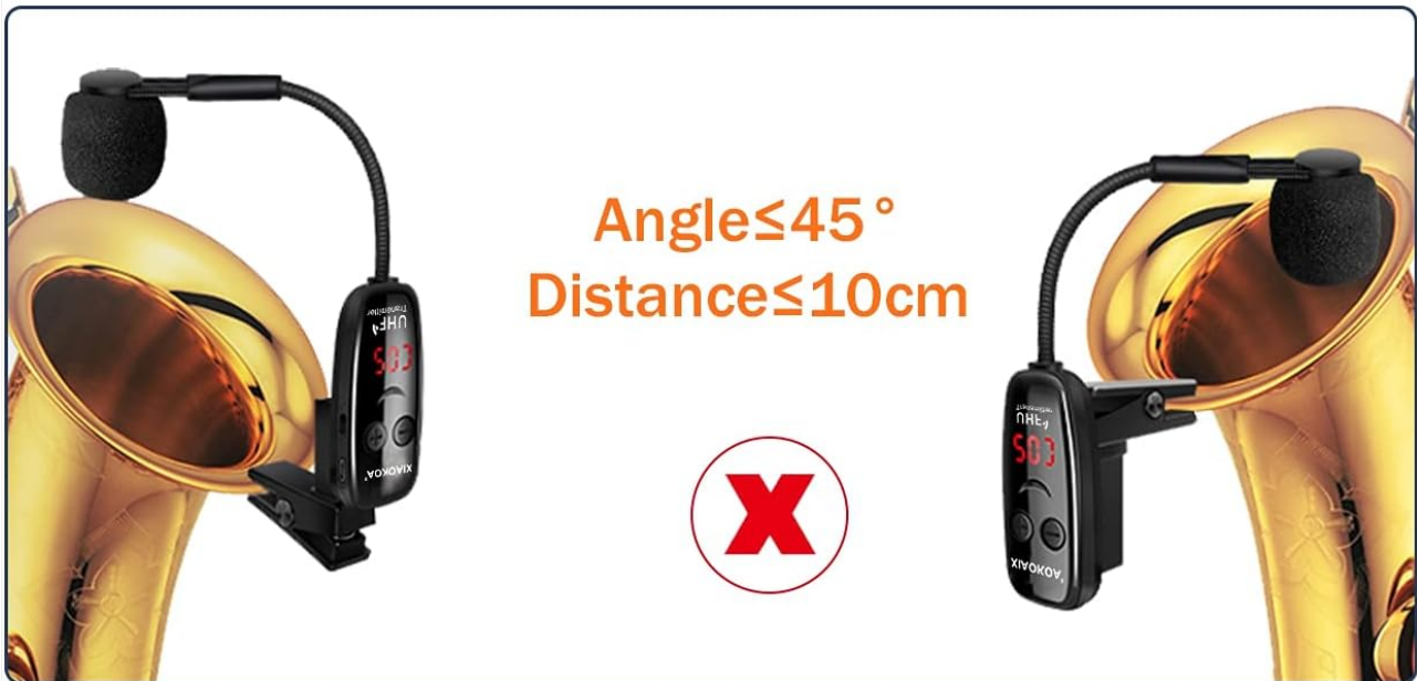
Image: Illustration showing the correct installation method for the transmitter on a saxophone, emphasizing the optimal angle ( \leq 45^\circ ) and distance ( \leq 10\text{cm} ) for the microphone head. An incorrect installation example is also shown.
