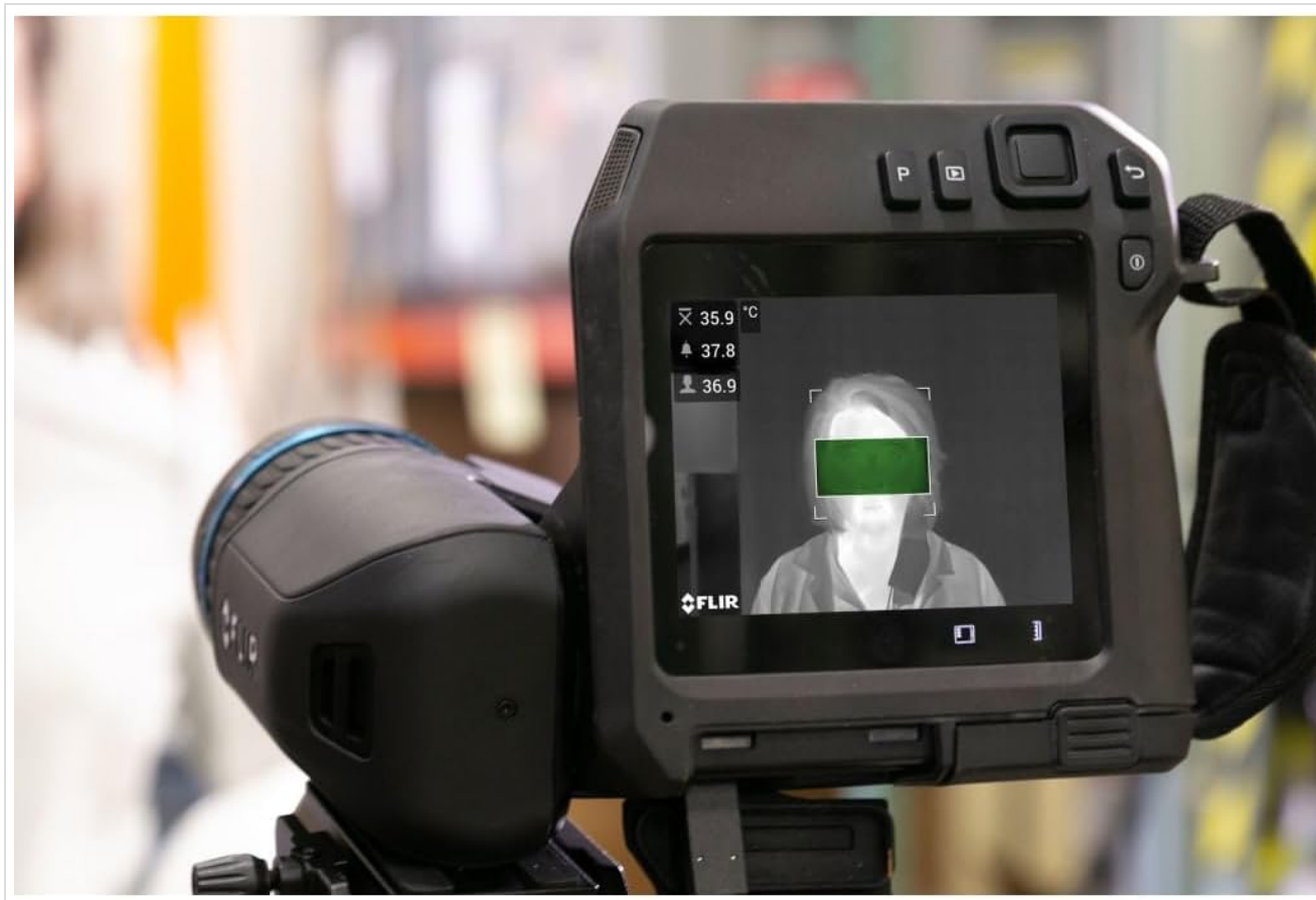
Figure 3: A detailed view of the FLIR T540-EST's integrated screen, showing real-time thermal data and a highlighted area for temperature assessment.
