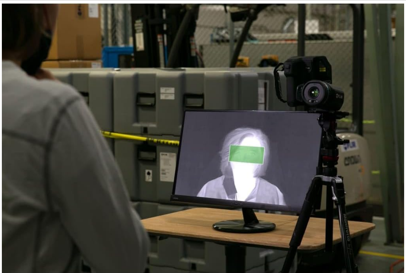
Figure 2: The FLIR T540-EST camera set up with an external monitor, displaying a thermal image of a person during a screening process.
