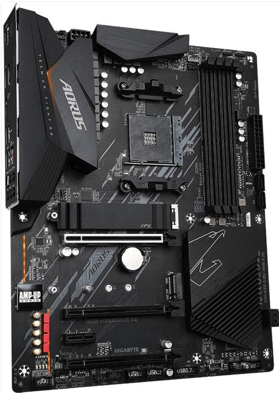
Figure 2.2: A detailed top-down view of the motherboard, showcasing the CPU socket (AM4), DDR4 DIMM slots, PCIe slots, M.2 slots with thermal guards, and various headers and connectors.
