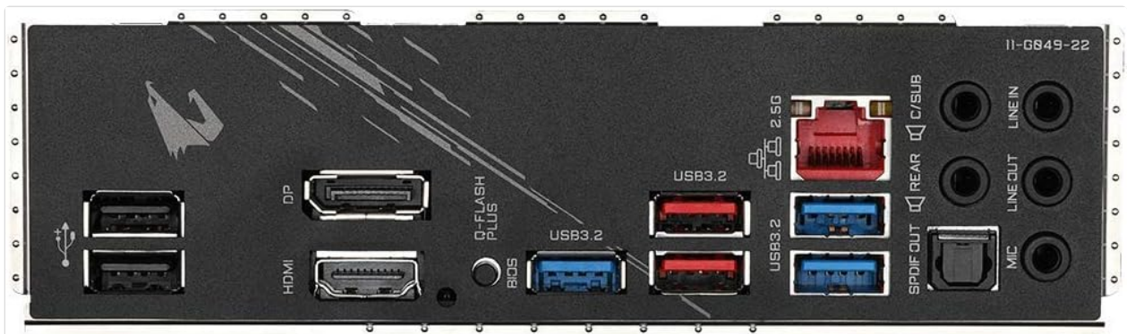
Figure 2.3: The rear I/O panel features multiple USB 3.2 ports, HDMI, DisplayPort, 2.5GbE LAN, audio jacks, and a Q-Flash Plus button for convenient BIOS updates.
