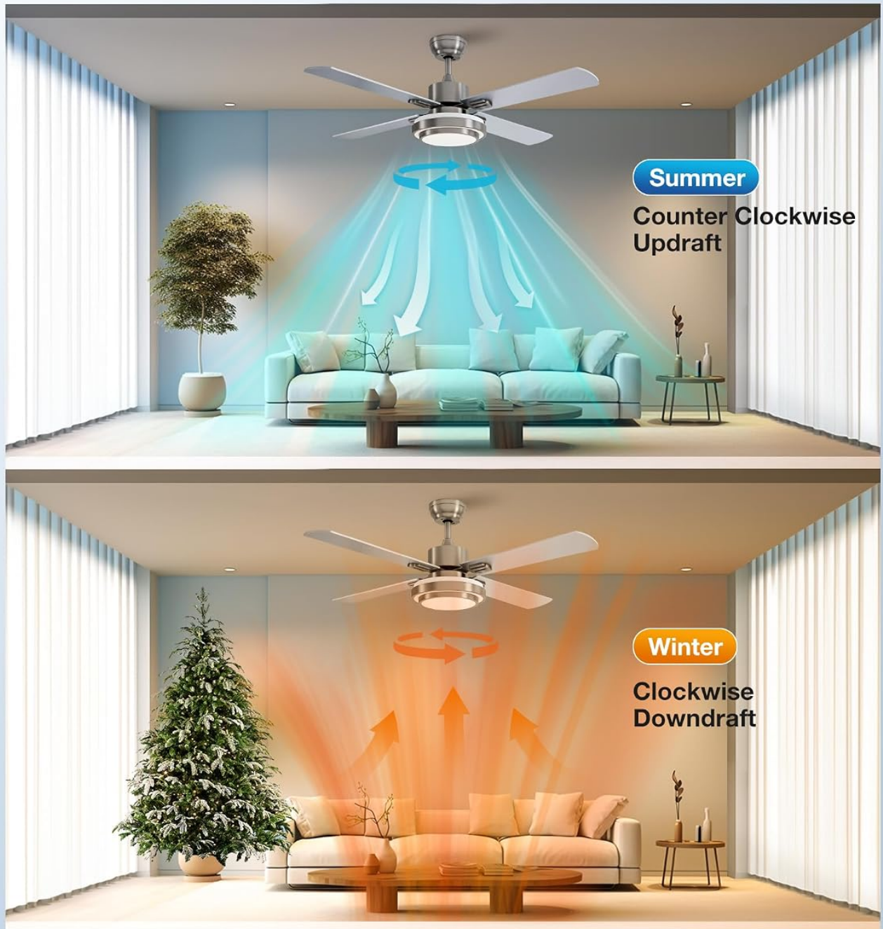
Figure 5: Fan airflow direction can be reversed for summer cooling (counter-clockwise updraft) or winter warmth (clockwise downdraft).
