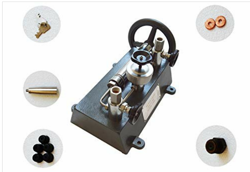
Figure 3.1: YJY-600 Pressure Calibrator with various accessories including seals and adapters.
