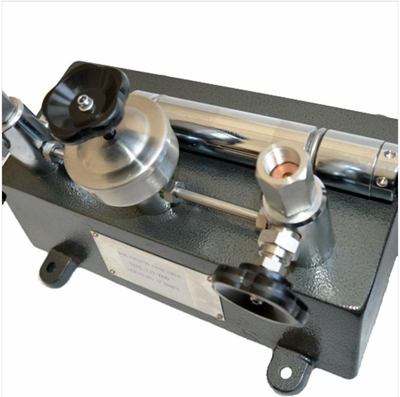
Figure 7.1: Detail of the fine-tuning handwheel and control valves for pressure regulation.
