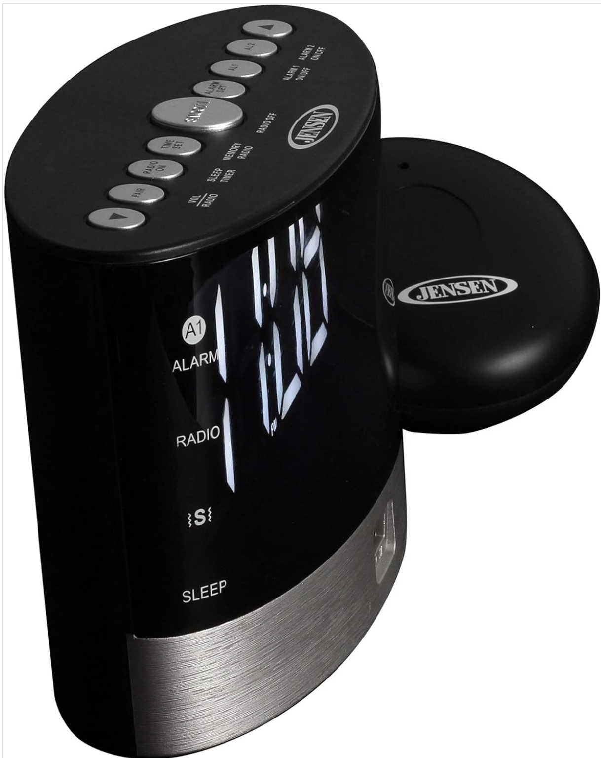
Figure 4: Top-down view of the JENSEN JCR-255 clock radio, showing the array of control buttons on the top panel and the under-pillow vibrator placed next to it. The clock display shows 11:11.
