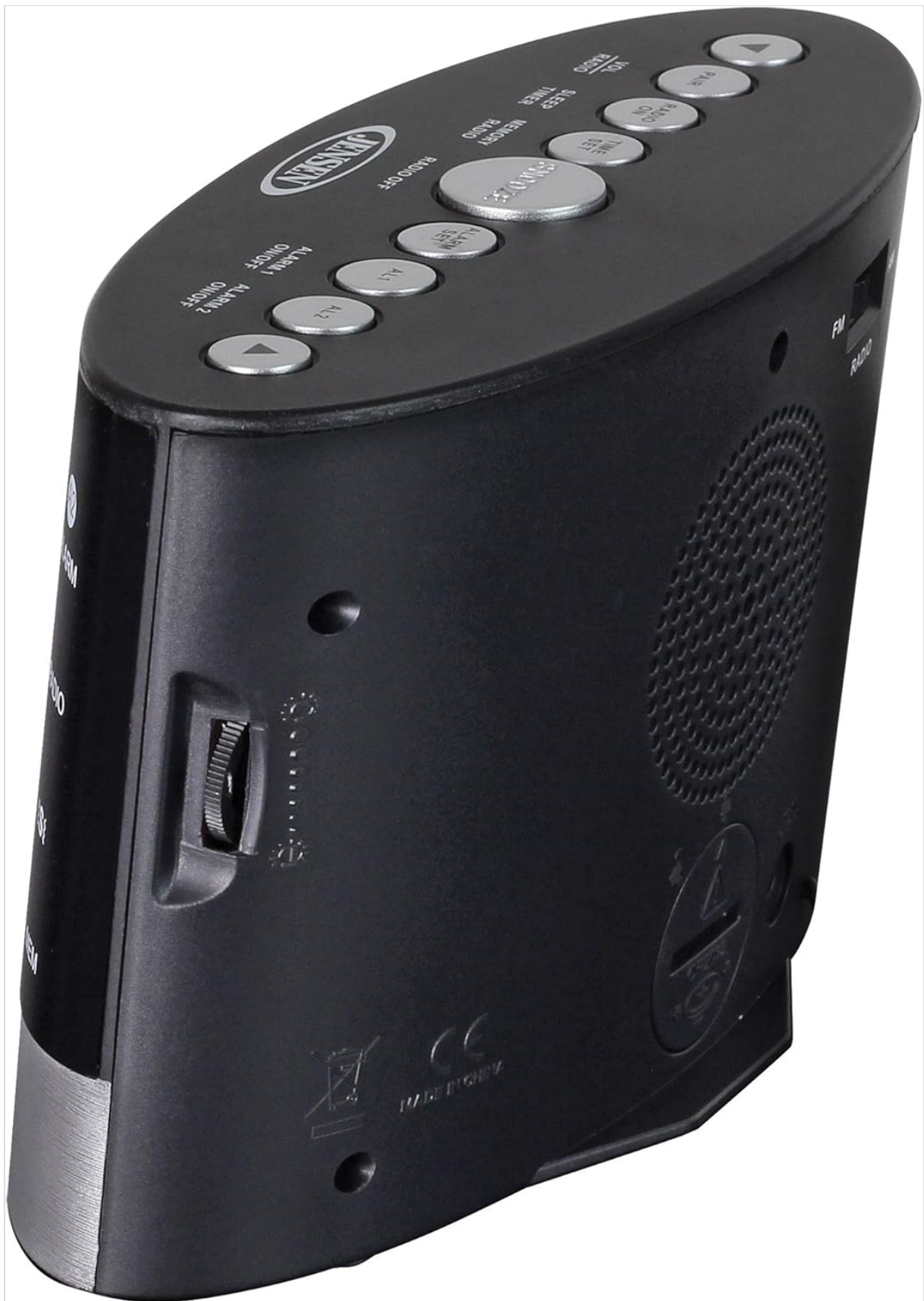
Figure 3: Side view of the JENSEN JCR-255 clock radio, showing the rotary dimmer control on the left side for adjusting display brightness. A speaker grille is visible on the right side.
