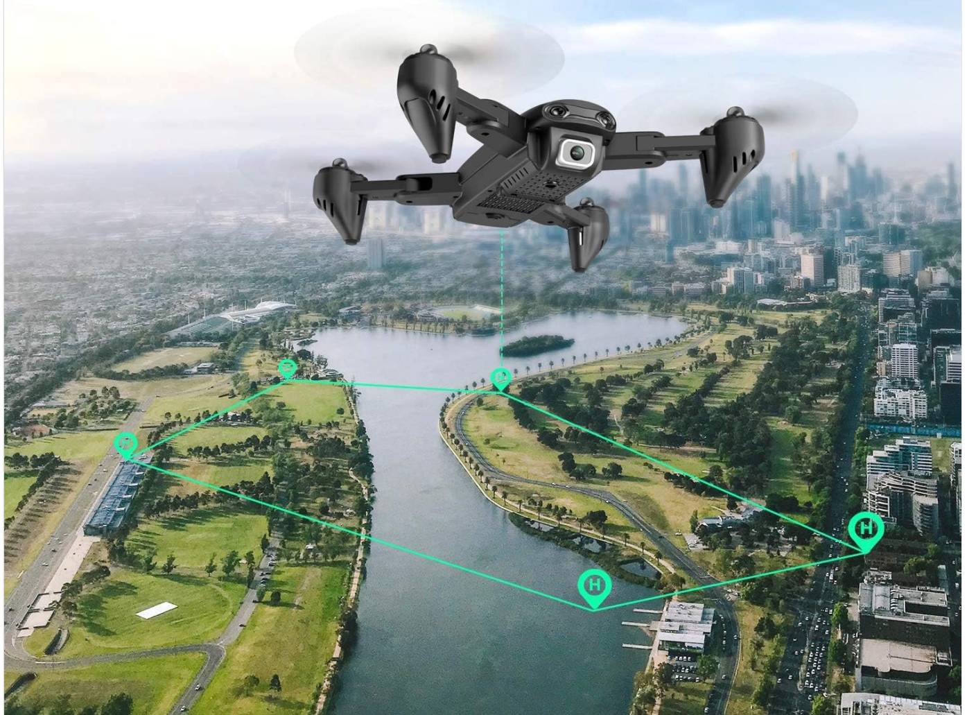
Figure 6.4: The Waypoint Fly feature allows the drone to follow a pre-defined path.
