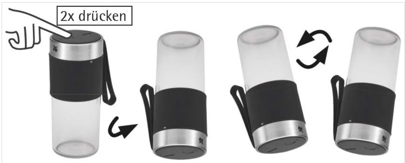
Image: Operational diagram showing the sequence: press the button twice, then invert and gently shake the mixer for optimal blending.
