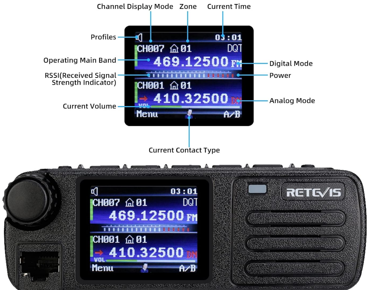
Figure 3: Large TFT Screen and Visual Operation.
