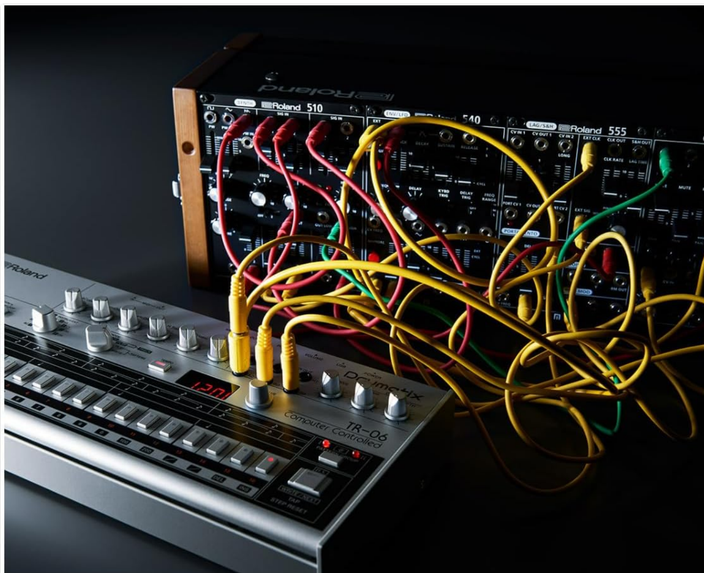
Figure 5: The TR-06 integrated into a modular synthesis environment, showcasing its trigger connectivity.
