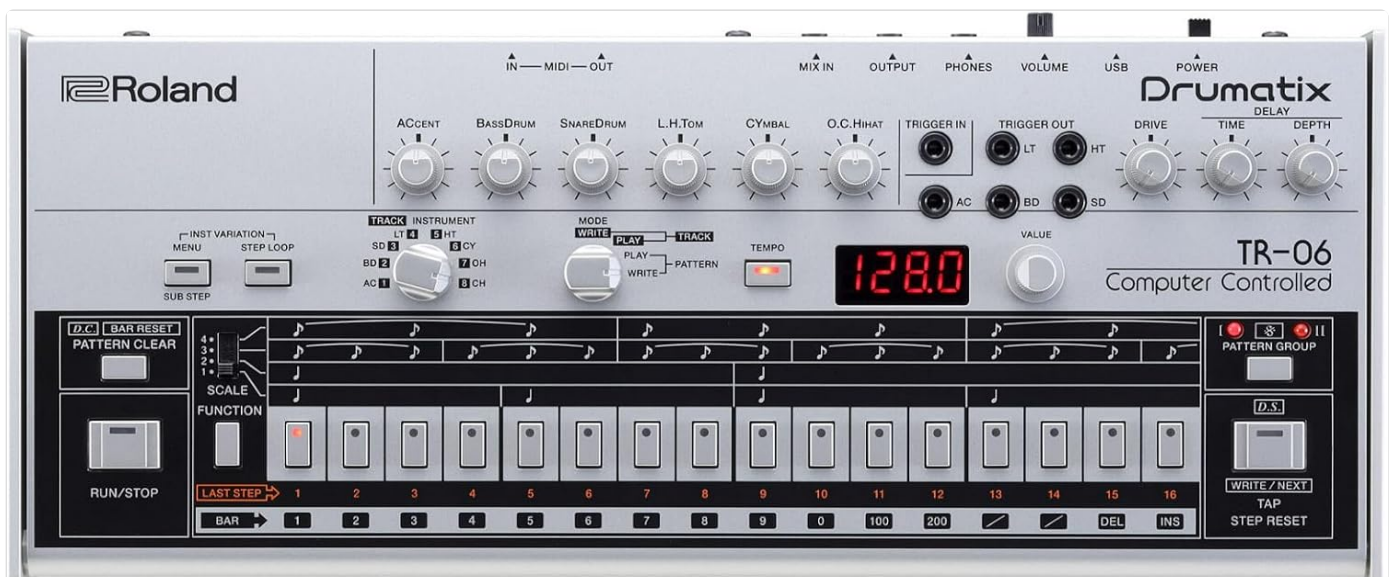
Figure 3: Front panel of the TR-06, displaying instrument controls, sequencer steps, and display.
