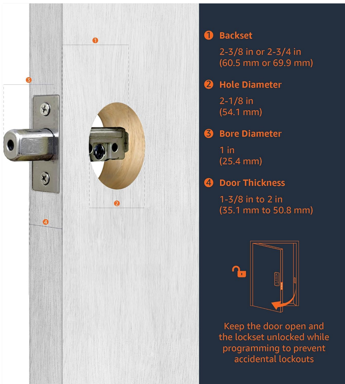
Figure 5.2: Guide for measuring door dimensions.
