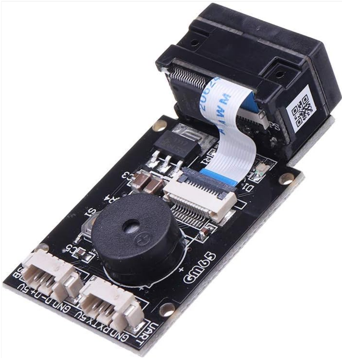
Figure 4.1: Top-down view of the ZOYOSI GM65 Barcode Reader Module, showing the scanner head, buzzer, and connection ports.
