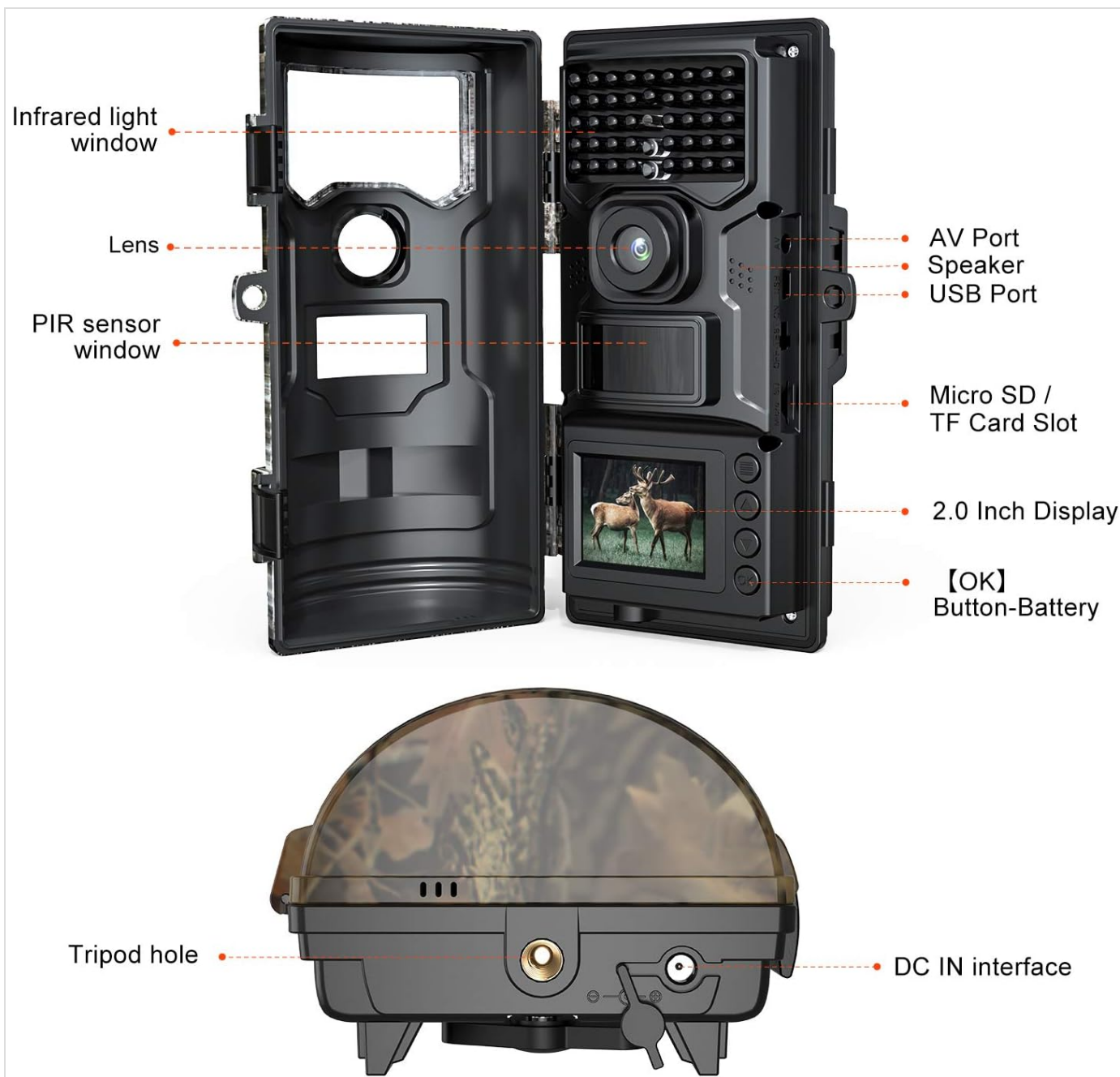
Figure 1: WiMiUS H7 Trail Camera Component Diagram. This image displays the camera with its front cover open, highlighting key parts such as the infrared light window, lens, PIR sensor window, 2.0-inch display, Micro SD/TF card slot, AV port, speaker, USB port, tripod hole, and DC IN interface.
