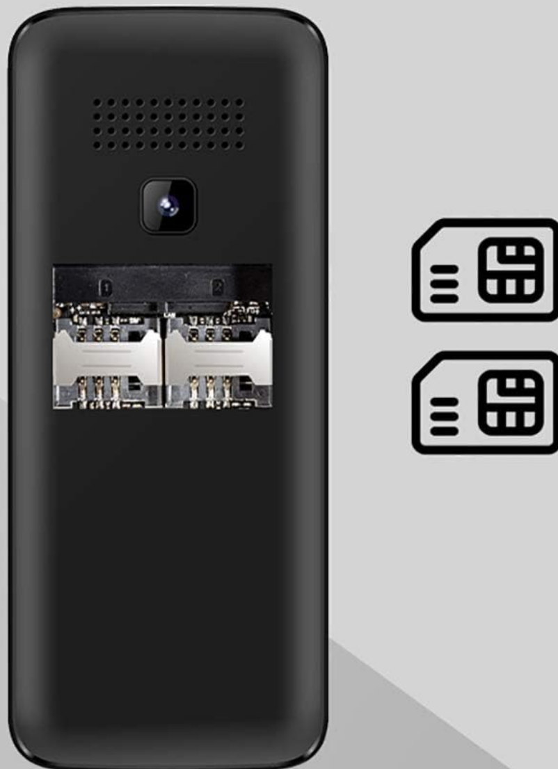
Image: The back of the UNIWA E1801 phone with the cover removed, clearly showing the two SIM card slots and an illustration of two SIM cards.
