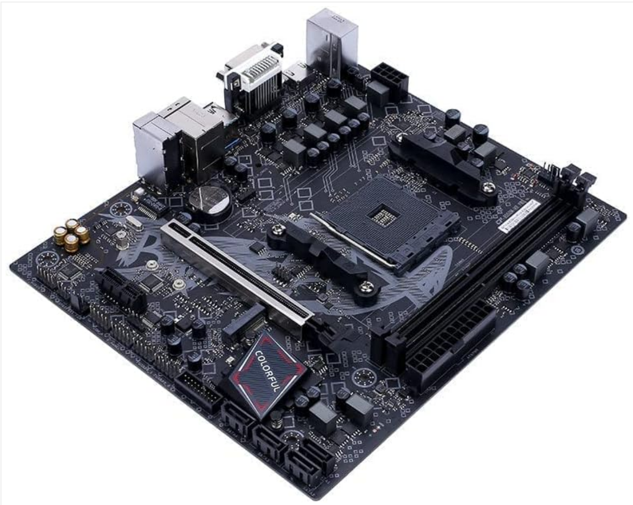
Figure 2: Angled view of the motherboard, providing a clearer perspective of the CPU socket, DDR4 memory slots, and power connectors.
