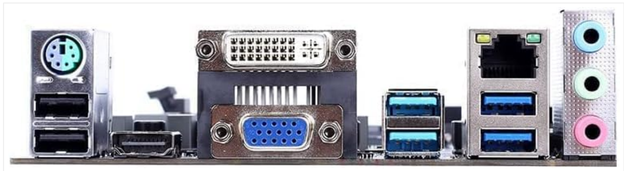
Figure 3: Rear I/O panel connectors, including PS/2, USB, video outputs (VGA, DVI, HDMI), LAN, and audio jacks.
