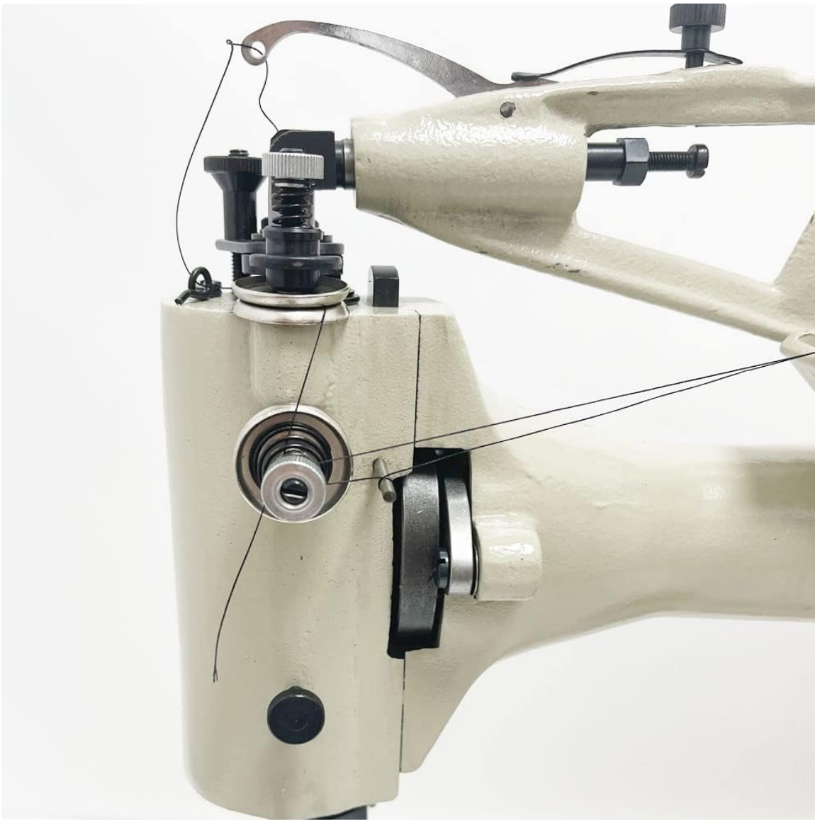
Image: Side view of the machine head, illustrating the complete upper threading process down to the needle.
