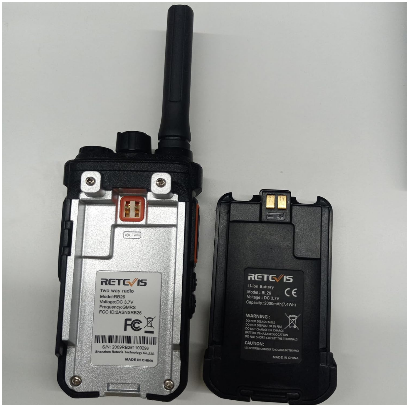
Image: The rear view of the Retevis RB26 radio with its battery compartment open, displaying the internal contacts, alongside the separate 2000mAh Li-ion battery ready for installation.
