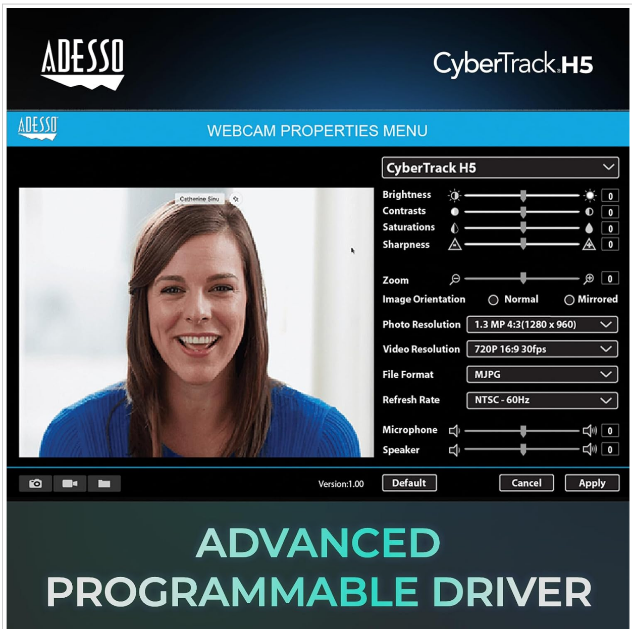
Image 5.1: A screenshot of the webcam's advanced programmable driver interface, showing options for brightness, contrast, saturation, sharpness, zoom, image orientation, resolution, file format, and microphone/speaker settings.
