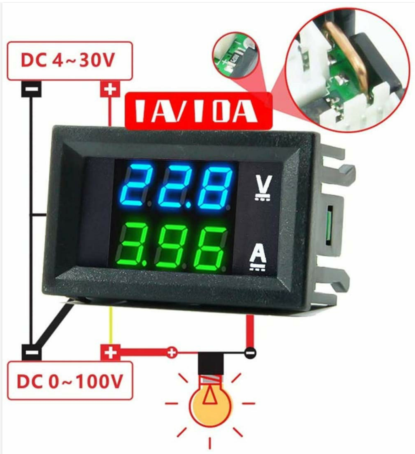
Image 5.1: Detailed wiring diagram for the diymore voltmeter ammeter. It illustrates the connections for the meter's power supply (DC 4-30V) and the circuit being measured (DC 0-100V, 0-10A load).
