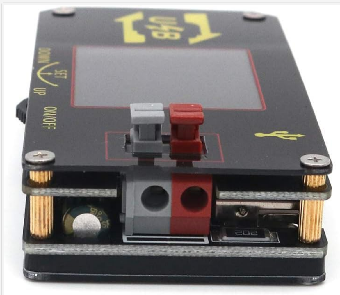
Figure 7: Close-up side view of the DollaTek XY-UDP module, showing the screw terminals and a control button.
