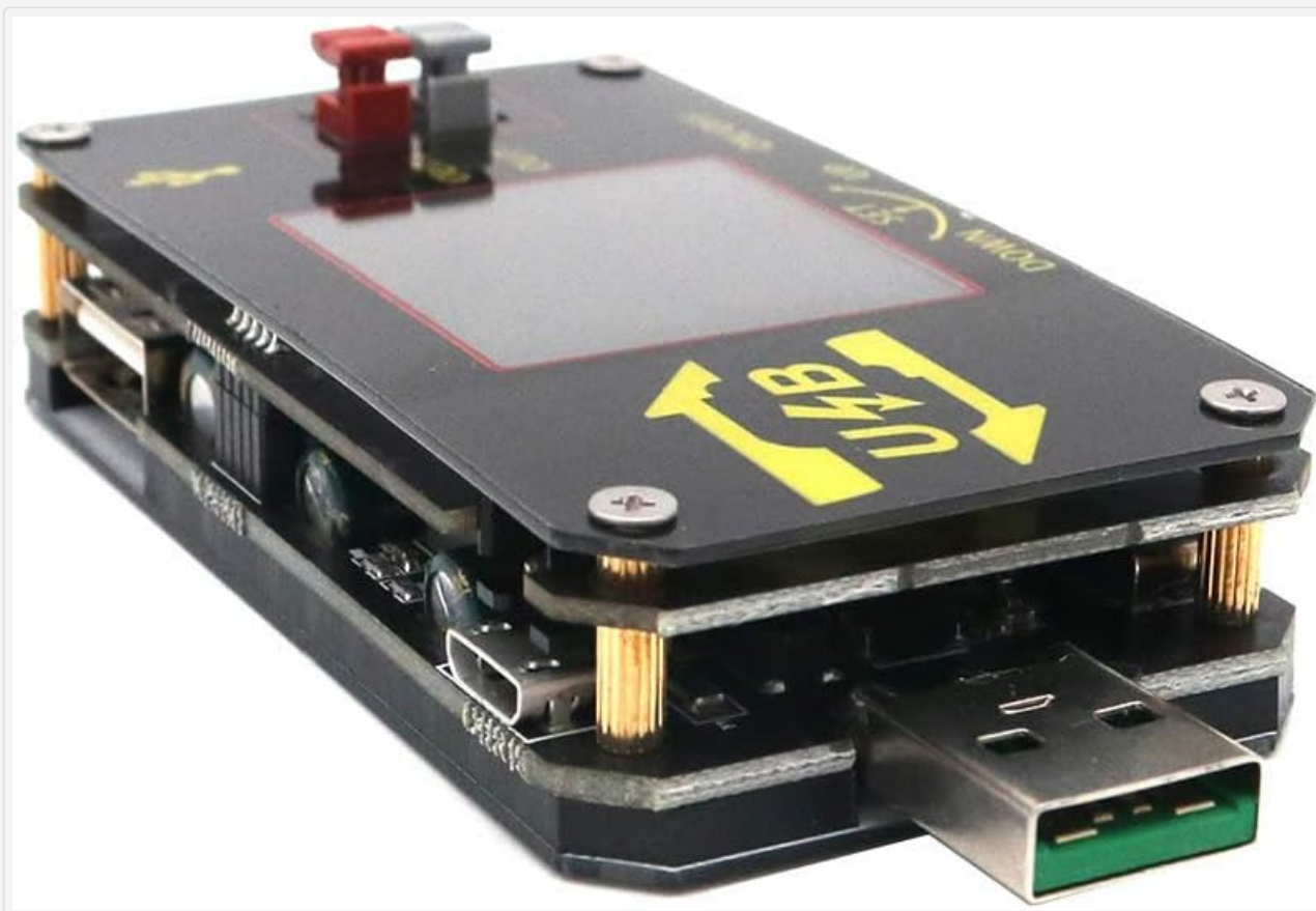
Figure 9: Angled view of the DollaTek XY-UDP module, showing the USB-A input and output ports from a different perspective.
