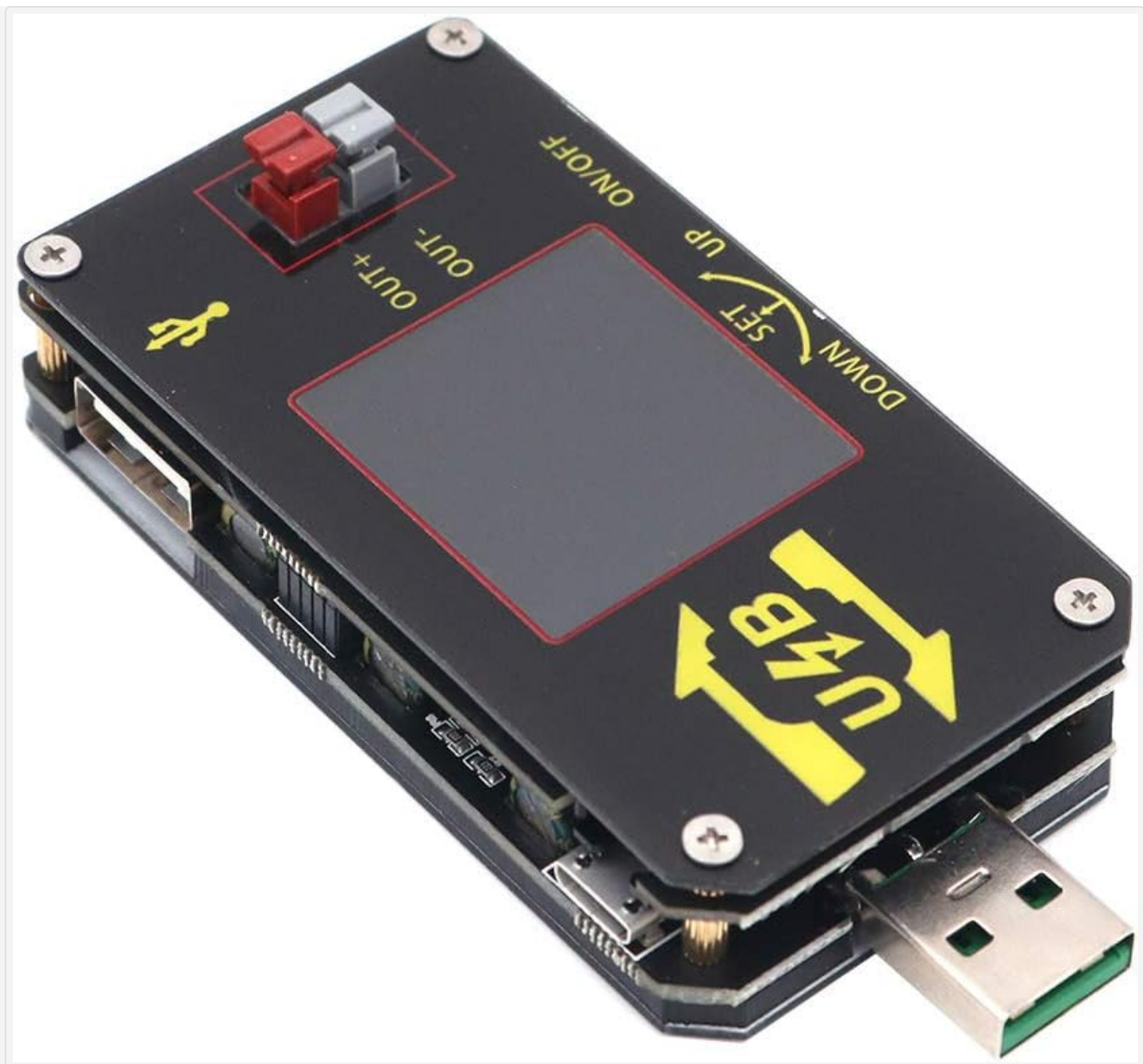
Figure 1: Angled view of the DollaTek XY-UDP module, showing the USB-A input, USB-A output, screw terminals, and LCD screen.
