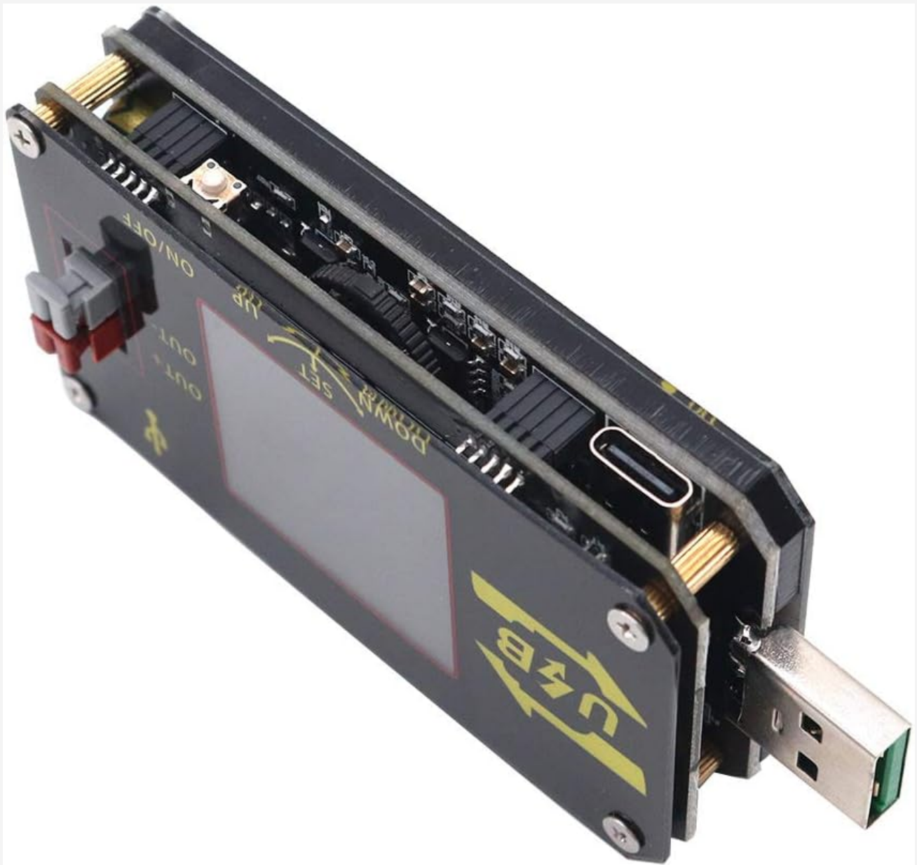
Figure 3: Side view of the DollaTek XY-UDP module, showing the USB-C input and USB-A output ports.
