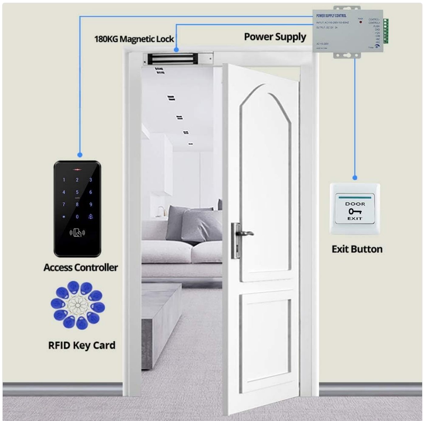
Figure 2.2: Diagram illustrating the interconnected components of the access control system, showing the access controller, magnetic lock, power supply, exit button, and RFID key cards in a typical door setup.
