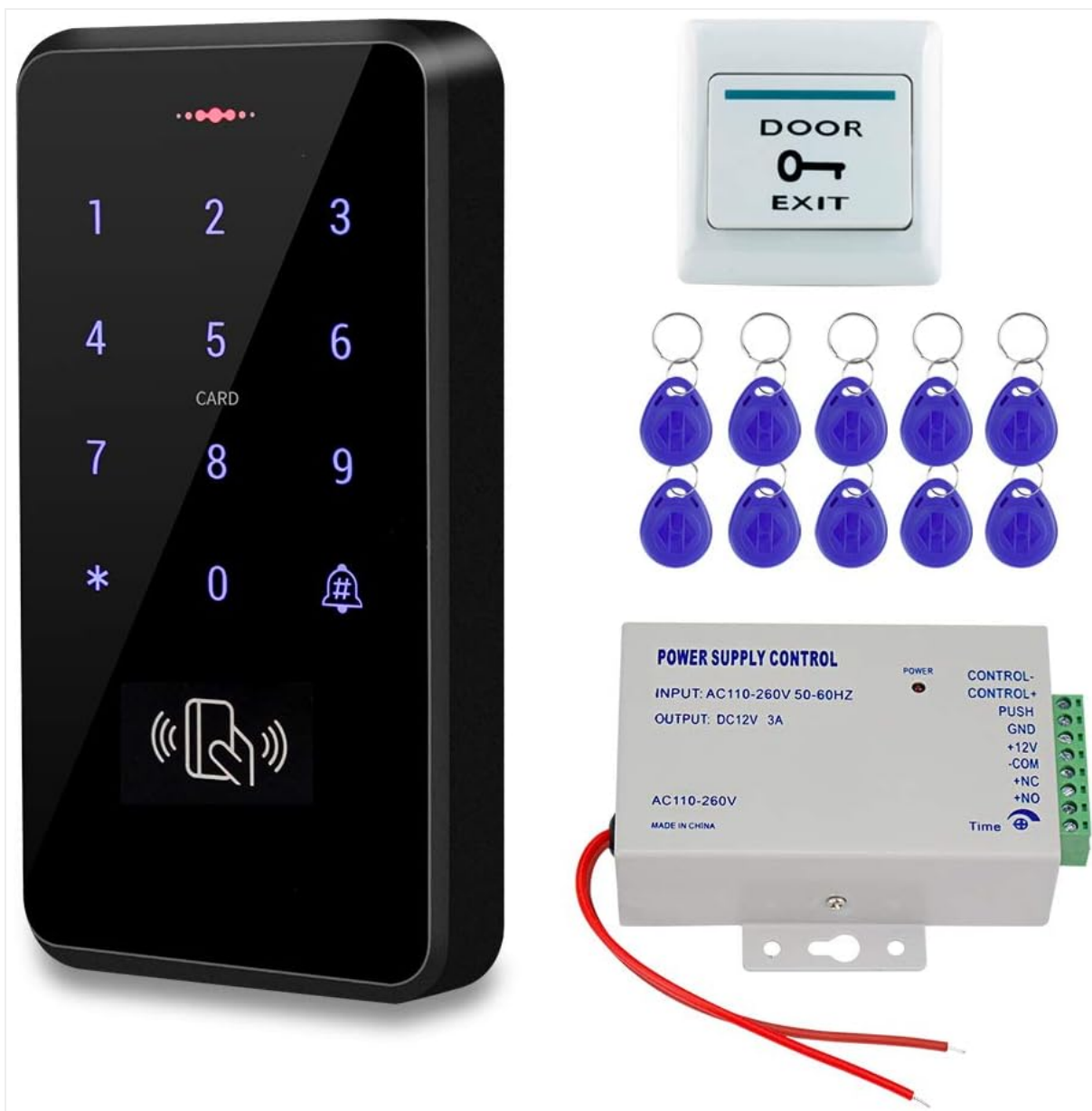
Image 1: Overview of the Diginex HFeng Outdoor Door Access Control System Kit, showing the RFID keypad, power supply, door exit button, and 10 RFID keyfobs.
