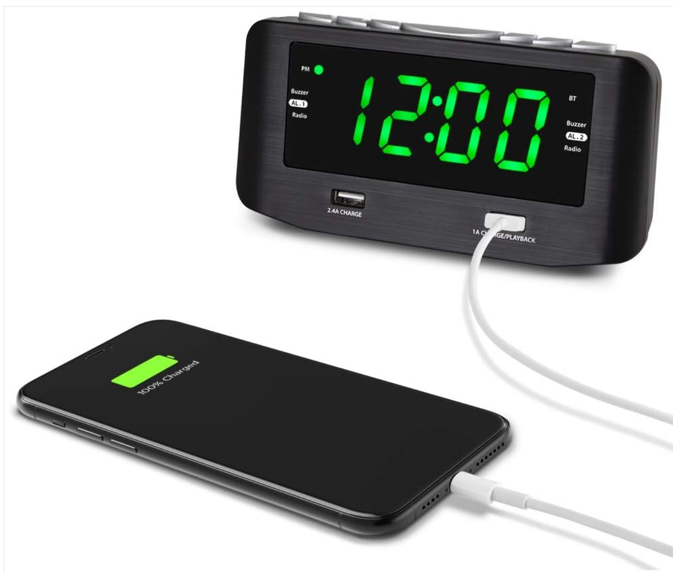
Figure 4: A smartphone connected to the 1A USB port for charging and potential MP3 playback.
