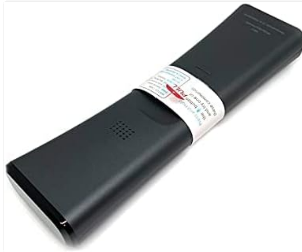
Figure 2: Back view of the remote, indicating the battery compartment location.
