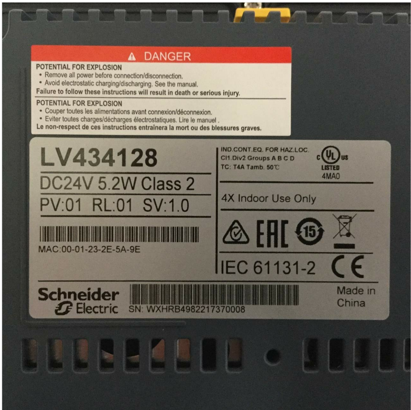
Figure 2.6: The rear of the LV434128 module, displaying critical safety warnings, electrical specifications (DC24V 5.2W), and regulatory compliance markings.
