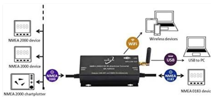
Image 2.1: Basic connection diagram showing the QK-A032-AIS connected to NMEA 2000 devices, an NMEA 0183 device, a PC via USB, and wireless devices via WiFi.
