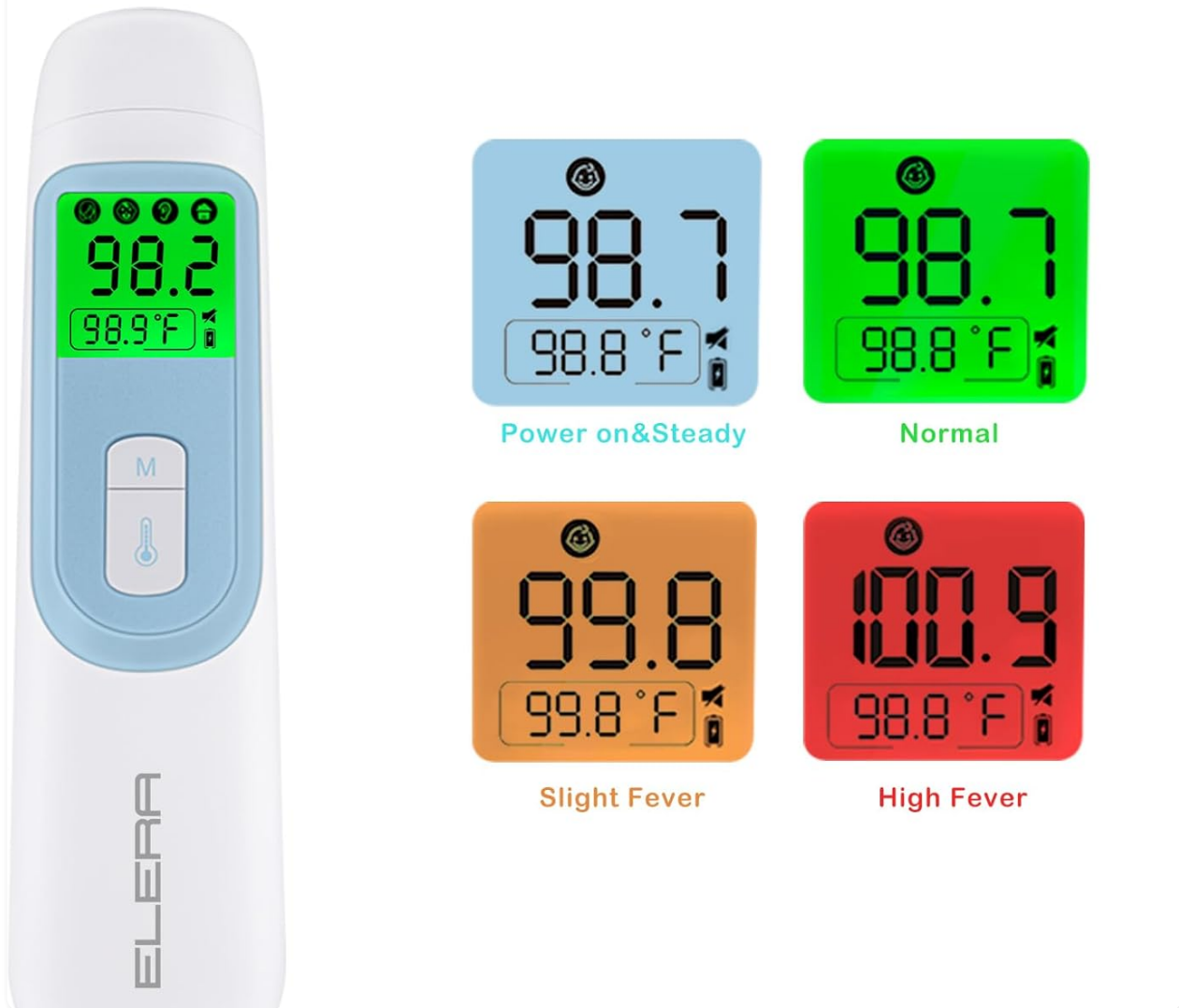
Image 4.4: The thermometer's display showing the four different backlight colors corresponding to temperature ranges.
