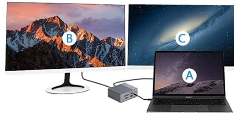
Figure 5: Illustration of display modes for macOS (mirror mode) and Windows (mirror and extended modes) using the docking station.
