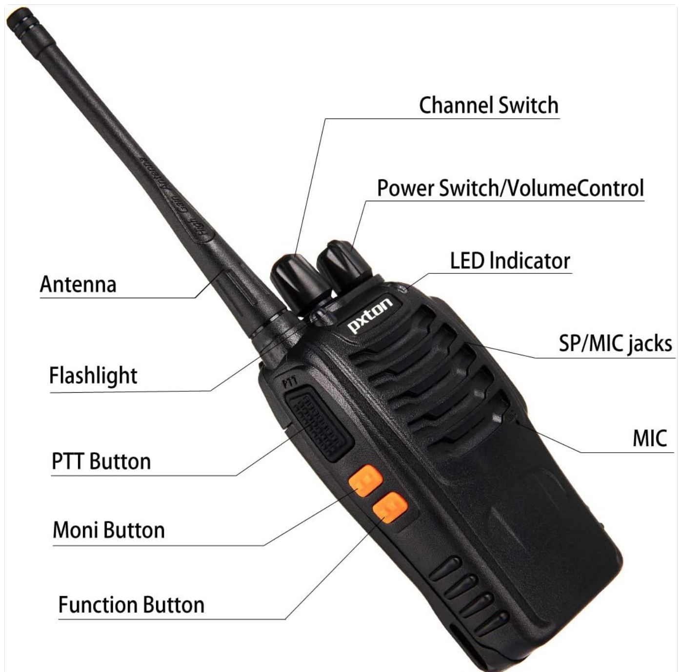
Figure 2: Labeled diagram of the pxton walkie talkie components.
