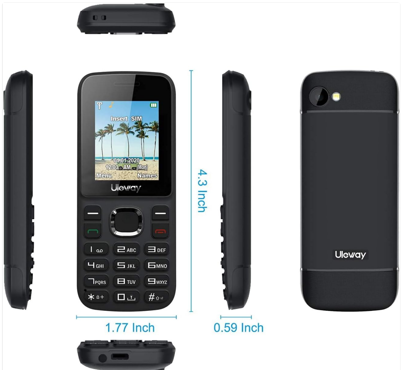
Figure 7.1: Physical dimensions of the Uleway W180 phone.
